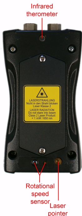
Figure 34: Rotation speed and temperature sensor, laser pointer
