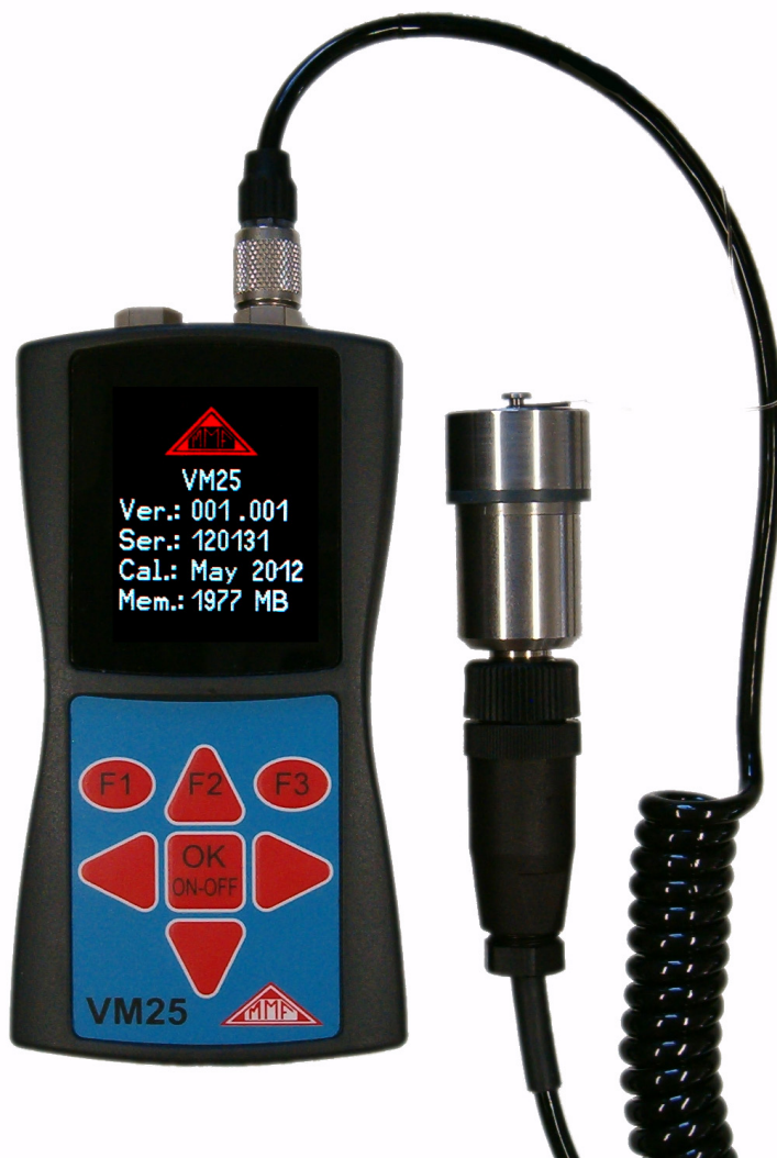
Figure 1: VM25 with vibration sensor
