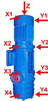
Figure 14: Measuring Points on Machines with Vertical Rotors
